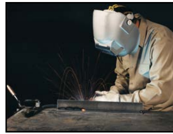
STT® using CO 2 and .045 in. solid wire. Note reduced spatter and fume.
